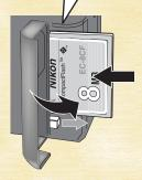
After inserting the memory card and making sure • that it is properly seated, close the slot cover.
